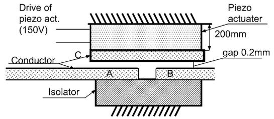
Fig. 2: Mechanical switchgear using piezoelectric device.
