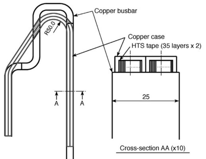
Fig. 2. Additional busbars with HTS tape conductors on the side of the copper busbar.
