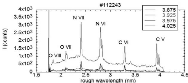
Fig. 1 EUV spectra measured with SOXMOS for the discharge #112243. N<sub>2</sub> gas was injected at  $t=3.8 - 3.9$ s.
