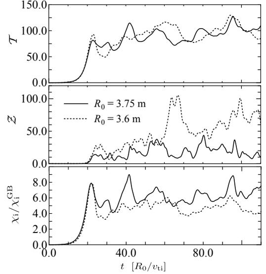
Fig. 1: Time evolutions of  $\mathcal{T}$ ,  $\mathcal{Z}$  and  $\chi_i / \chi_i^{\text{GB}}$  resulting from the gyrokinetic simulations. Solid curves correspond to the case for  $R_0 = 3.75$  m, and dotted curves for the vacuum magnetic configuration with  $R_0 = 3.6$  m.
