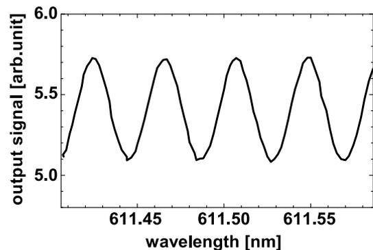
Fig. 2: Output signal of the interferometer as a function of dye laser wavelength.
