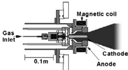
Fig. 1 Schematic of an MPD arcjet
