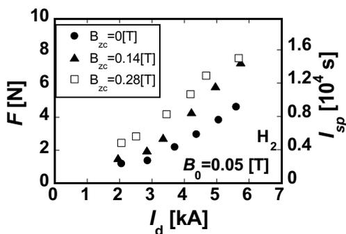
Fig. 2 Dependence of thrust and specific impulse on discharge current with and without magnetic nozzle applied to the MPD outlet.
