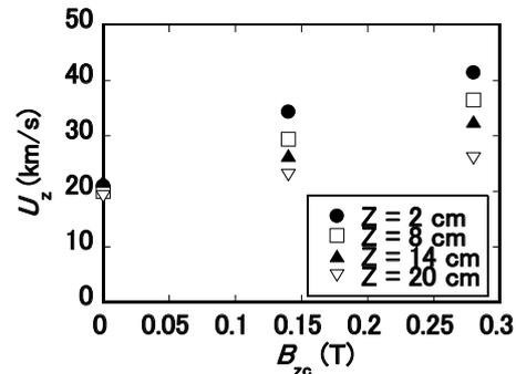
Fig. 3 Dependence of plasma flow velocity on the applied magnetic nozzle field intensity.
