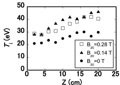
Fig. 4 Axial profiles of ion temperature with various applied magnetic nozzle field intensity.
