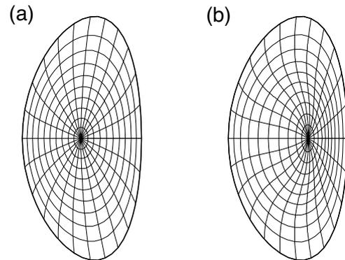
Fig. 2. Magnetic surfaces of (a) vacuum equilibria and (b) 2% averaged beta equilibria of a new configuration.
