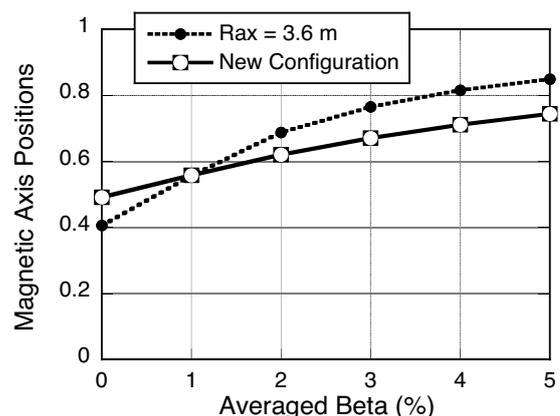
Fig. 3. Relative positions of magnetic axis with increased beta.
