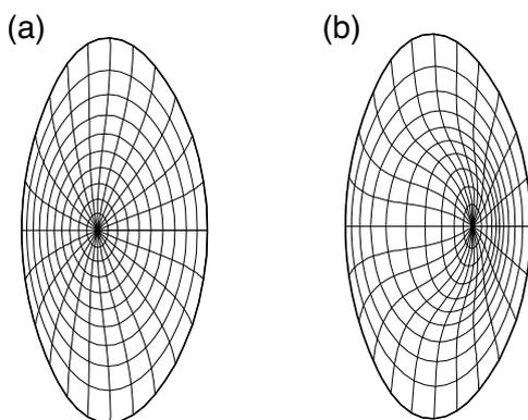
Fig. 1. Magnetic surfaces of (a) vacuum equilibria and (b) 2% averaged beta equilibria of LHD inward shifted configuration.
