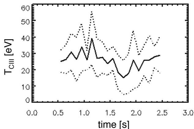
Fig. 1. Time evolution the Carbon ion temperature measured by Doppler broadening of the CIII line (464.7 nm) in LATE. The dotted lines indicate the range of  $\pm 1\sigma$ .
