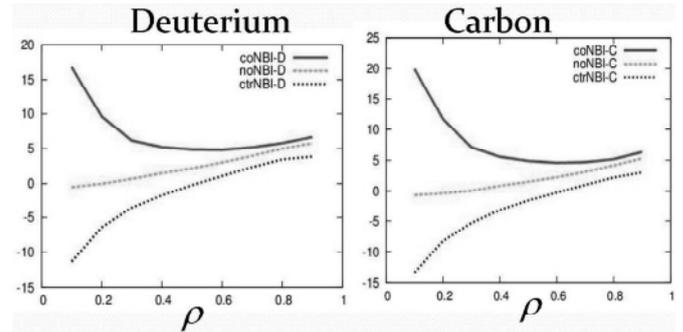
Fig.1 Calculated ion flow velocities  $\langle Bu_{||a} \rangle$  [T·km/s]. The co- and counter-injection shots and a case without the external momentum input are compared.
