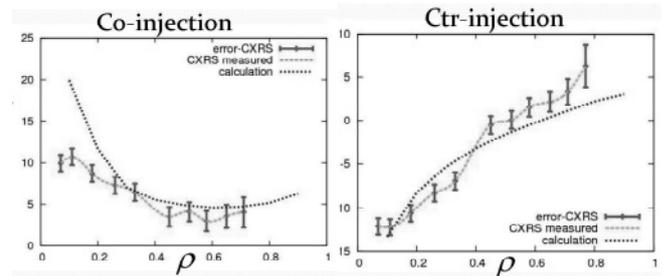
Fig.2 The calculated and measured  $\langle Bu_{||a} \rangle / B$  [km/s] of the  $C^{6+}$  ions.
