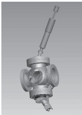
Fig. 29. 3-D figure of the beam section pattern detector
