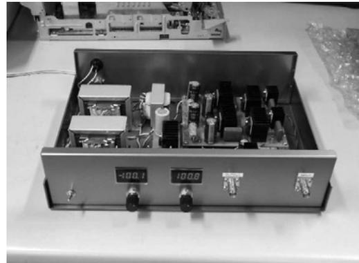
Fig. 2. High voltage pulse amplifier.
