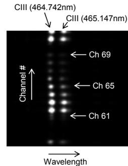
Fig.3. CCD image of CIII (464.742, 465.147 nm) at channel 61 to 69, indicated with red spots in Fig.1.
