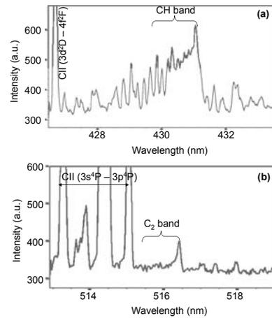
Fig. 2. (a) CH band and (b) C<sub>2</sub> band detected with the 2D spectrometer at the channels viewing the divertor plates (#121178, #121184).
