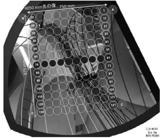
Fig. 1. Viewing area of the divertor spectrometer system. The dashed (yellow) circles represent spatial location of each channel of optic fibers with channel number.
