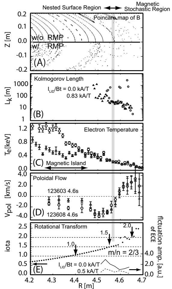
Fig. 1: Profile of the Kolmogorov Length (B), the electron temperature (C), the poloidal velocity (D) and the rotational transform estimated by HINT2 and the mode amplitude profile (E) are shown.
