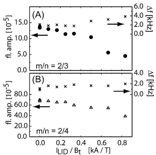
Fig. 2: Mode amplitude and spectral width of MHD activities with  $m/n = 2/3$  (A),  $2/4$  (B) as a function of the externally applied magnetic field.
