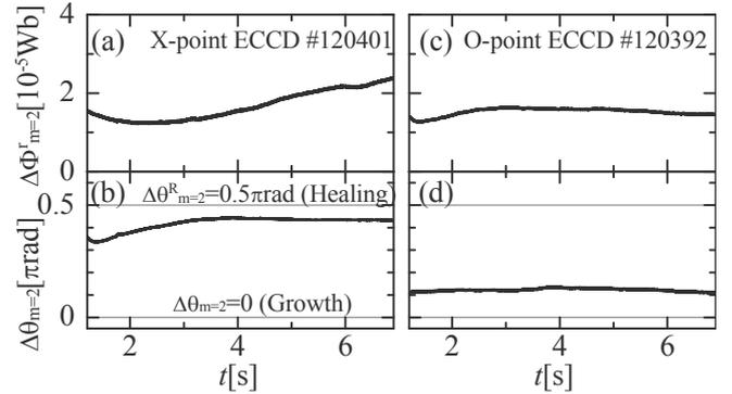
Fig.2 Time evolution of (a, c) plasma response field with  $m/n=2/1$  mode and (b, d) phase difference between RMP and plasma response field. (Left) X-point ECCD. (Right) O-point ECCD
