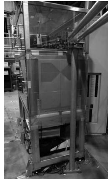
Fig. 2: The bow-tie antenna installed outside the vacuum vessel
