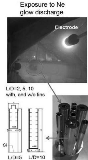
Fig. 2: Photographs of plasma exposure and cylinder with and without fins
