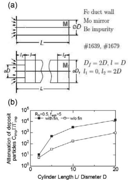
Fig. 1: (a) Structure of cylinder with and without fins [2] (b) Attenuations of impurity particles at the bottom of the cylinders.
