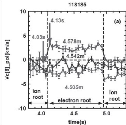
Fig.1 Temporal evolution of plasma rotation (poloidal) showing a reversal in the rotation from negative (ion root) to positive (electron root) in the plasma edge region ( $R > 4.54$  m) in the plasma discharge 118185.
