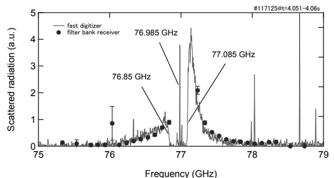
Fig. 1. Fine CTS spectrum measured by the CTS receiver with the fast digitizer for LHD#117125. The CTS spectrum measured by the filter bank receiver is plotted for the comparison. The magnetic configuration of LHD is  $B_t = 2.75$  T and  $R_{ax} = 3.6$  m.
