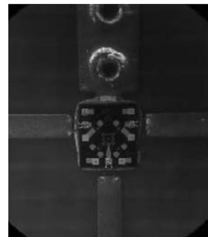
Fig. 4 MMIC mixer bonding on PCB.
