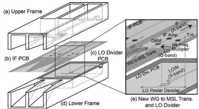
Fig.1 Conceptual diagram of HMA with internal LO.
