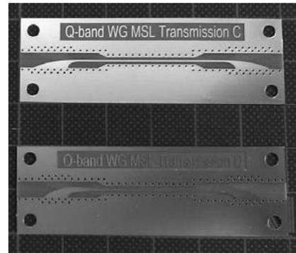
Fig. 2 PCB of 40 GHz waveguide to microstrip line transmissions.
