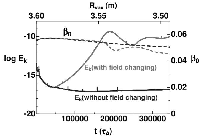
Fig. 1: Time evolution of kinetic energy ( $E_k$ , solid lines) of the  $n = 1$  component of the perturbation and axis beta ( $\beta_0$ , dashed lines) in the cases with and without the background field changing.
