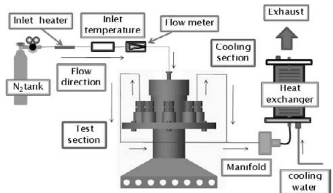
Fig.1 Experimental set up of gas cooling
