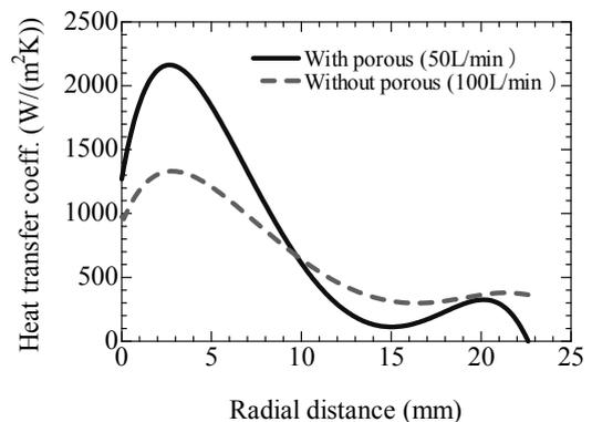
Fig. 2 Heat transfer coefficient in a radial direction
