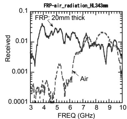
Fig.2 Frequency response of dipole antenna with/without the dielectric lamination.
