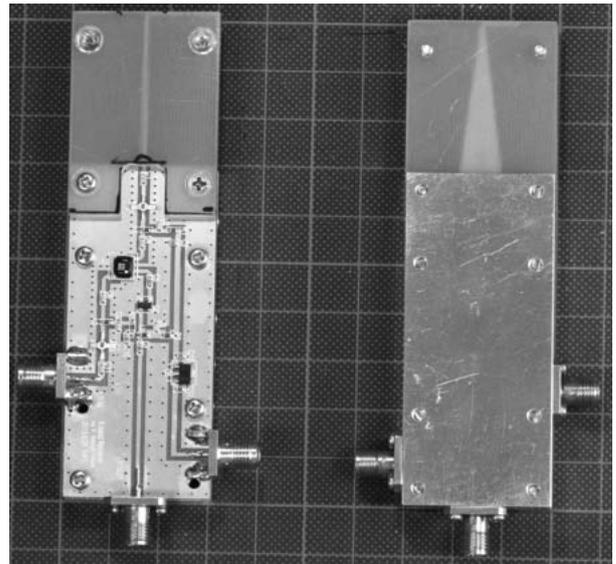
Fig. 1 Dielectric Laminated Dipole Antenna (DLDA).
