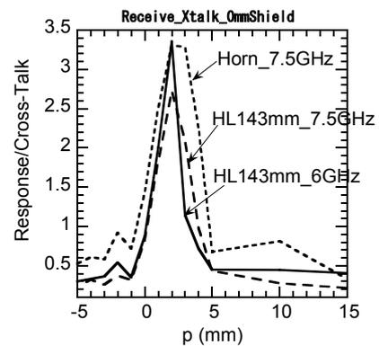
Fig. 3 Ratio of the response and the cross-talk in DLDA with shield as a function of distance ( $p$ ) between the shield and the dipole.
