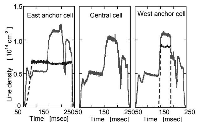
Fig.2 Temporal evolution of the line density in the east anchor, central and west anchor cells when direct ICRF powers are injected in both east and west anchor cells.
