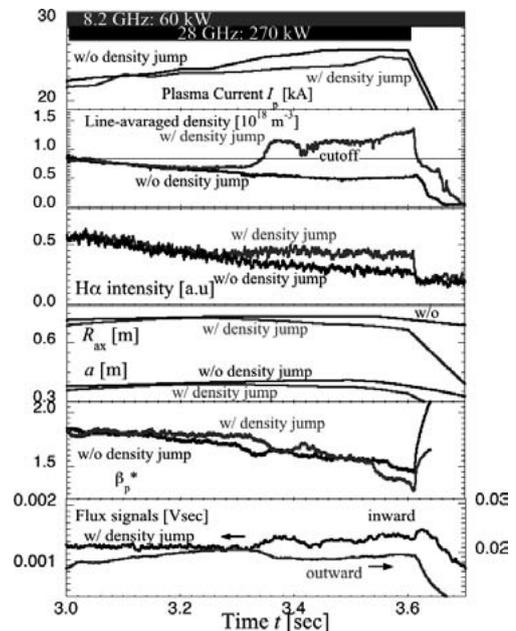
Fig.3: Time evolution of  $I_p$ , line-averaged density,  $H\alpha$  intensity,  $R_{ax}$ ,  $a$  and  $\beta_p^*$  w/ and w/o the density jump. Flux signals of inward and outward positions are also shown in the density jump case.
