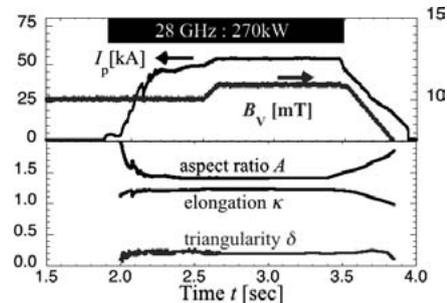
Fig.2: Time evolution of  $I_p$ ,  $B_v$ , aspect ratio  $A$ , elongation  $\kappa$  and triangularity  $\delta$  in the inner limiter-configuration.
