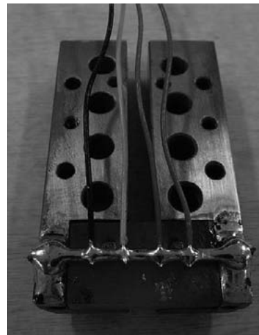
Fig. 2. Set-up status of Nb 3 Sn strand on sample holder. A new Nb 3 Sn strand was used.
