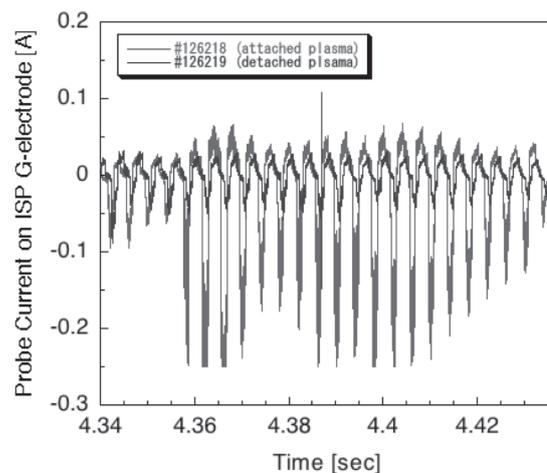
Fig. 2: Probe currents of the ISP guard electrode measured by using the fast reciprocating probe system at 4.5U port during an attached and a detached plasma discharges.
