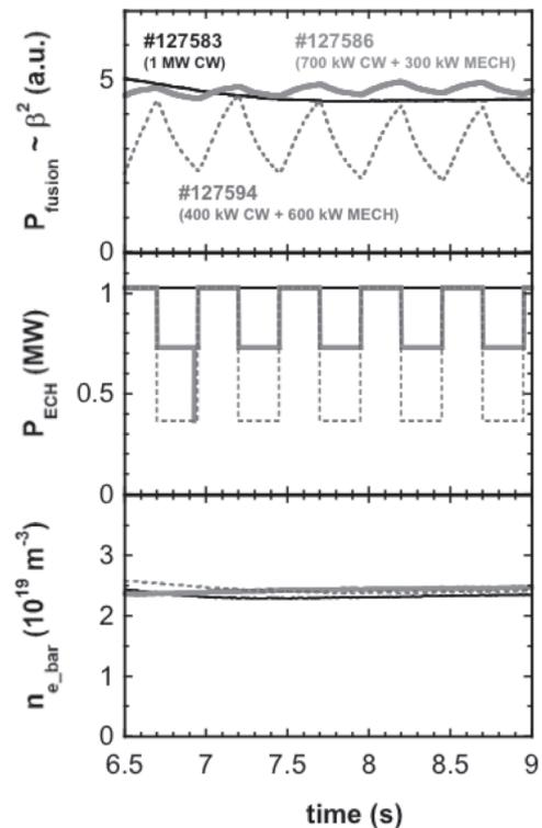
Fig. 2. Typical waveforms in discharges with, or without ECH modulation. From top to bottom, shown are the square of the plasma beta,  $\beta^2$  ( $\propto P_{fusion}$  in the fusion reactor), the ECH power,  $P_{ECH}$ , and the line-averaged electron density,  $n_{e\_bar}$ .
