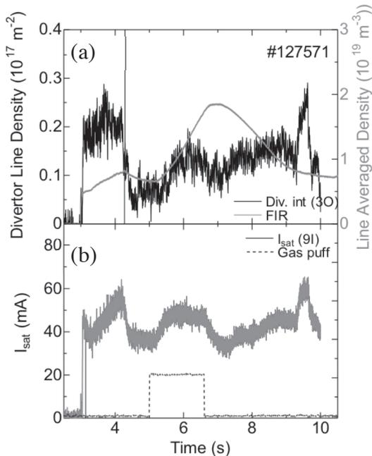
Fig. 1. Typical waveforms in an ECH complete detachment discharge, where (a) the divertor line electron density,  $n_{e\_div}$ , and the line-averaged electron density,  $n_{e\_bar}$ , (b) the ion saturation current measured on a divertor plate at the 9I port,  $I_{sat}$  (9I), and the gas flow pattern of the gas puffing are shown.
