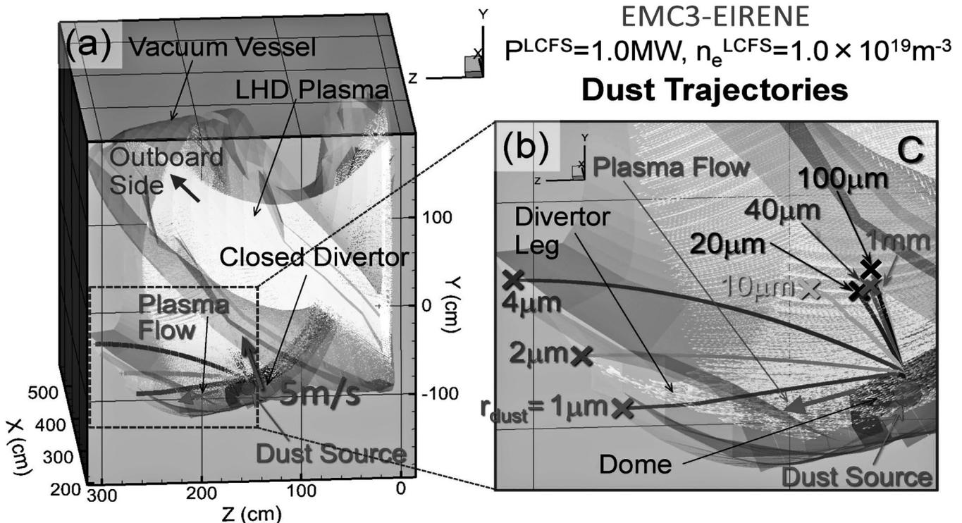
Fig. 1. An aerial view of the three-dimensional model of a LHD plasma and the vacuum vessel for dust transport simulation (a), and an enlargement view of the simulations of dust trajectories with various dust radii (b).
