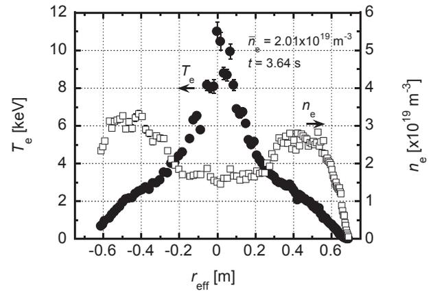
Figure 2. The radial profiles of  $T_e$  and  $n_e$  in a typical high  $T_e$  plasma with  $n_{e\_fir}$  of  $2 \times 10^{19} \text{ m}^{-3}$  produced using ECRH alone.
