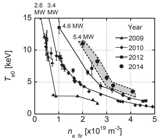
Figure 3. The map of simultaneously attained  $T_{e0}$  and  $n_{e\_fir}$  for ECRH discharges.
