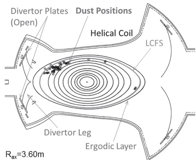
Fig. 2. The poloidal positions of the dusts observed with stereoscopic fast framing camera just before the plasma termination.
