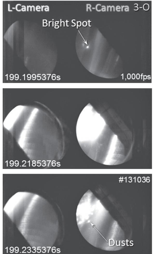
Fig. 1. Sequential stereoscopic images of a long pulse discharge observed with a fast framing camera installed in an outer port (3-O).
