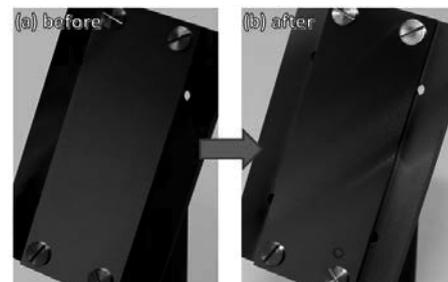
Fig. 2. Surface photo of the tungsten surface (a) before and (b) after exposure to the helium long pulse discharges.
