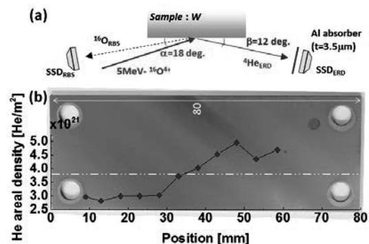
Fig. 3. (a) Geometry of the Oxygen probe beam ERD analysis and (b) Surface profile of the retained helium on the tungsten.
