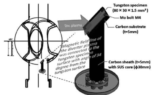
Fig. 1. Experimental set up of the plasma irradiation at divertor position in LHD.
