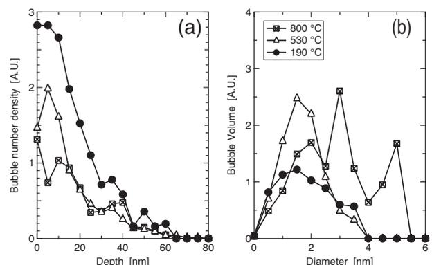
Fig. 2: Temperature dependence of (a) bubble depth distribution, and (b) bubble size distribution.
