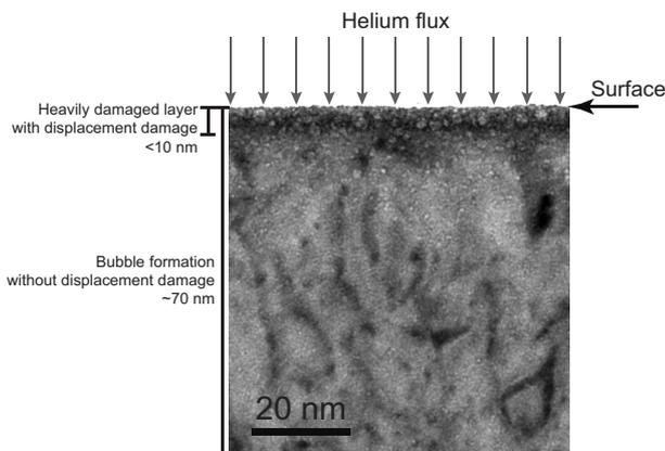
Fig. 1: Cross-sectional TEM image of the helium exposed tungsten at 800 °C
