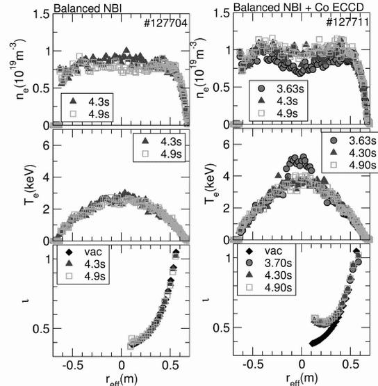
Fig.1: Profiles of the electron density (upper), the electron temperature (middle) and the rotational transform (lower) in plasmas sustained by balanced NBI (left) and sustained by balanced NBI and co ECCD (right)
