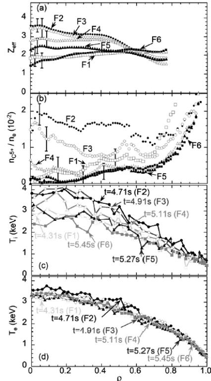
Fig.2 Profiles of (a)  $Z_{\text{eff}}$ , (b)  $n_{\text{C}^{5+}}/n_e$ , (c)  $T_i$  and (d)  $T_e$  in the six time frames of F1-F6.
