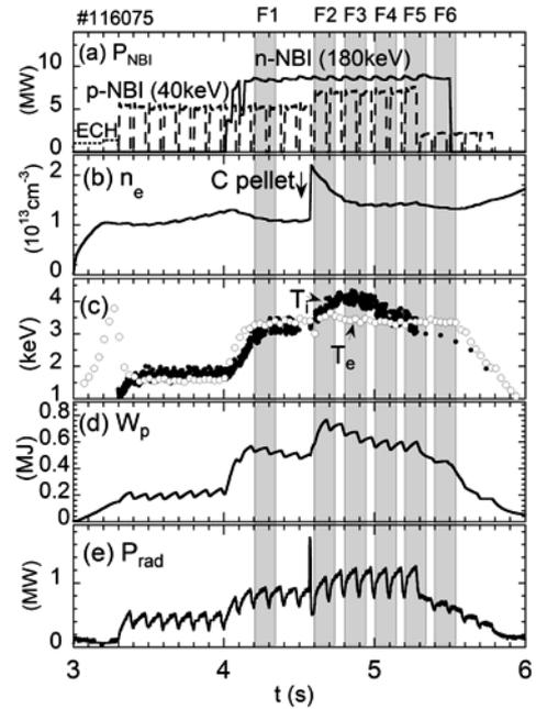
Fig.1 Time evolution of (a) NBI port-through power, (b)  $n_e$ , (c)  $T_e$  and  $T_i$ , (d) plasma stored energy  $W_p$  and (e) radiation power  $P_{\text{rad}}$ . Dashed areas indicate six time frames of F1-F6.
