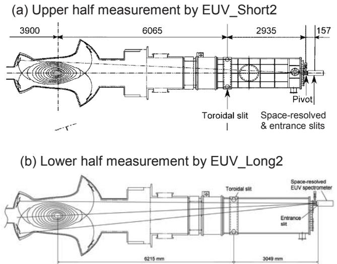
Fig.1 (a) EUV\_Short2 spectrometer for upper half profile measurement (b) EUV\_Long2 spectrometer for lower half profile measurement.
