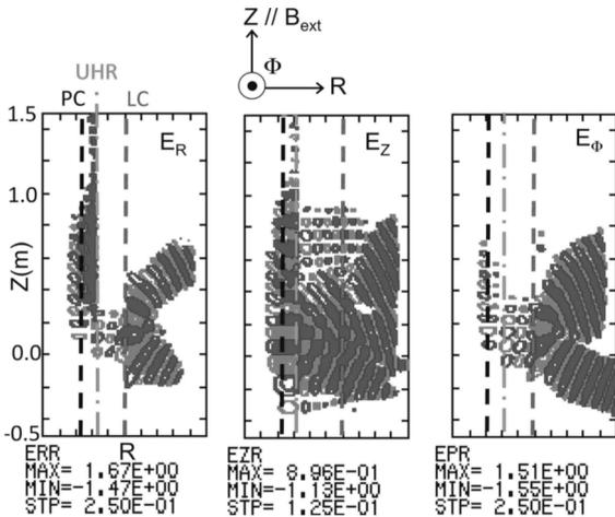
Fig.1: Contour maps of electric field components of 5GHz wave launched from right lower side as a linear polarized X-mode dominant wave.
