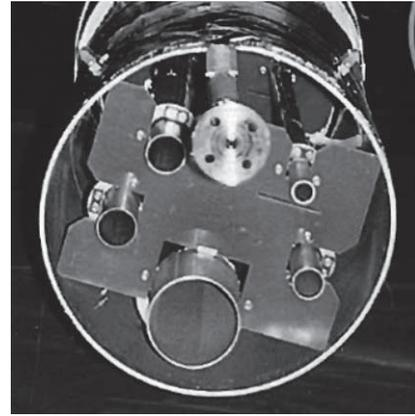
Fig. 1. Photograph of the cross section of the target cryogenic line
