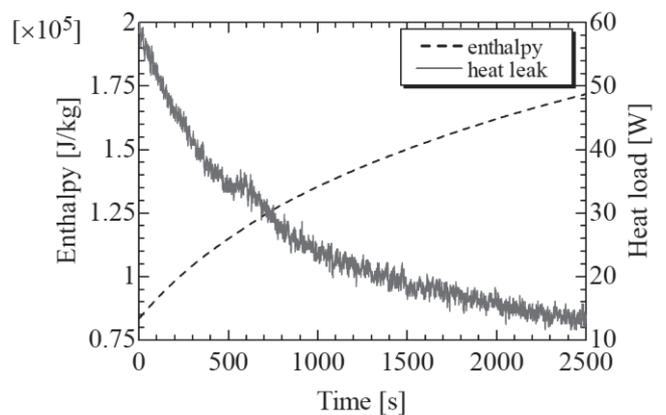
Fig. 3. Enthalpy change calculated with HEPAK and estimated heat leak.
