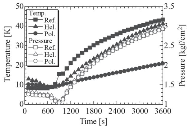
Fig. 2. Temperature and pressure profiles in the transfer tube after the inlet and outlet valves were closed.
