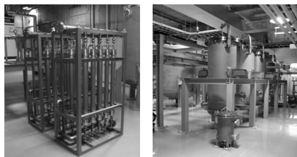
Fig. 2. Photos of the polymer permeable membrane module set for the purge gas detritiation system (left) and the molecular sieves beds for the vacuum gas detritiation system (right).
