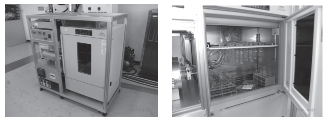
Fig. 2. Photos of tritium sampling system ; the appearance of tritium sampling system (left) and the water bubbler system in the incubator (right).
