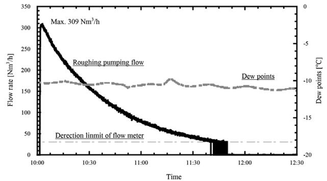
Fig. 1. The variation of the roughing pumping flow rate of LHD vacuum vessel.
