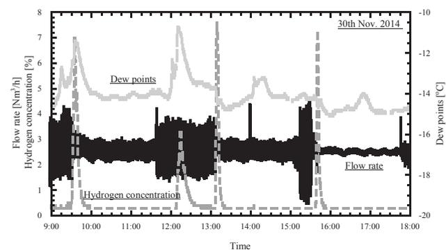
Fig. 3. The example of the variation of hydrogen concentration and flow rate on Sunday, 30<sup>th</sup> Nov. 2014.
