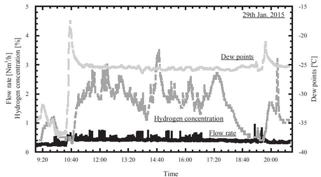
Fig. 2. The example of the variation of hydrogen concentration and flow rate under plasma experiments at 29<sup>th</sup> Jan. 2015.
