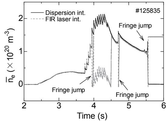
Fig. 2: Measurement results of the FIRlaser interferometer and the dispersion interferometer of a pellet injected discharge.
