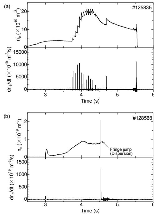
Fig. 3: Measurement results of (a) ice pellets and (b) impurity pellets injected plasmas.
