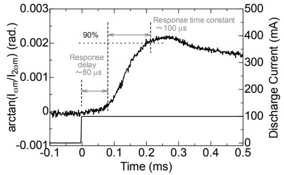
Fig. 1: A Temporal behaviour of the CO<sub>2</sub> laser dispersion interferometer.
