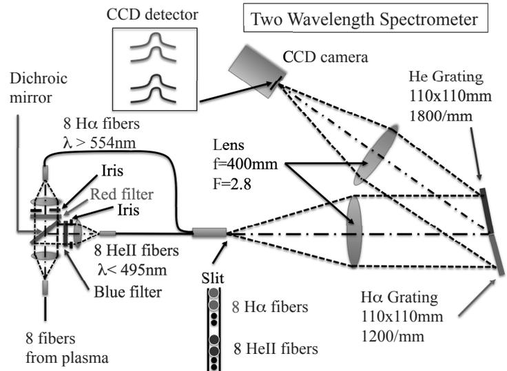
Fig. 1: Two-wavelength spectrometer for helium/hydrogen density ratio measurement with charge exchange spectroscopy.
