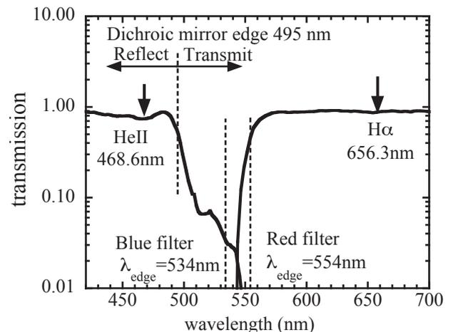
Fig. 2: Transmission of HeII channel and  $H_{\alpha}$  channel through the dichroic mirror plus red and blue filter in the two-wavelength spectrometer system.
