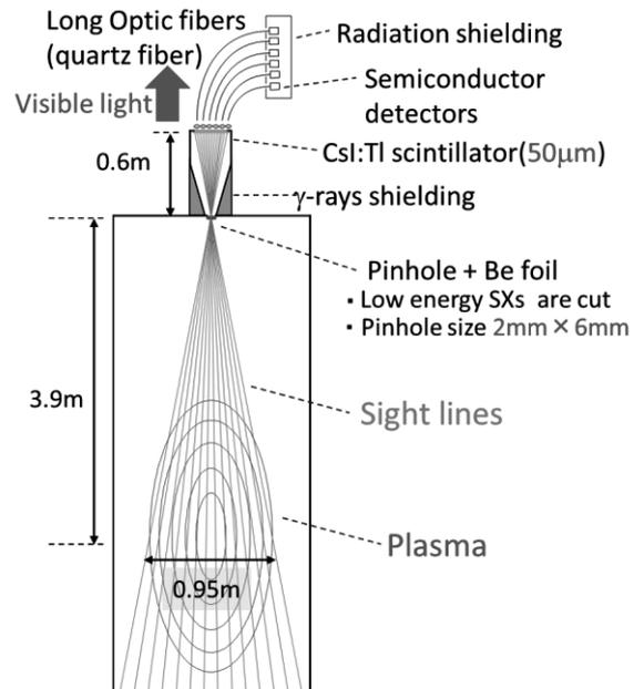
Fig. 1. The schematic view of the design of the diagnostic is shown. Sight lines viewing a plasma cross section are shown as green lines.
