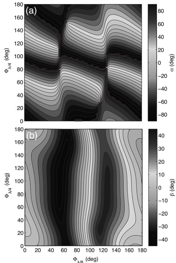
Fig. 2: Polarization state (a)  $\alpha$  and (b)  $\beta$  as a function of polarizer rotation angles ( $\Phi_{\lambda/8}$ ,  $\Phi_{\lambda/4}$ ) for the combination of the optimally-designed  $\lambda/8$ - and  $\lambda/4$ -type polarizers.
