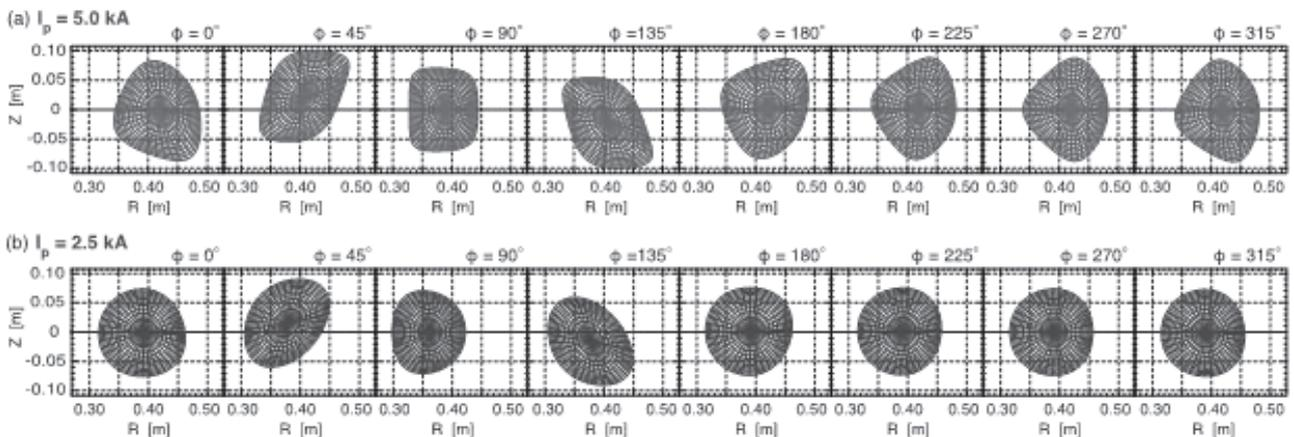
Fig. 2 Comparison of the flux surfaces between two cases of plasma current  $I_p = 5$  kA and 2.5 kA calculated with the VMEC code in its free-boundary mode.  $I_{PS} = 10$  kA in both cases. The PS coils are located between  $\phi = 0^\circ$  and  $\phi = 180^\circ$ .
