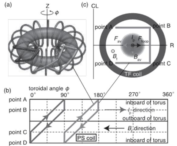
Fig. 1 Location of the parallelogram-shaped saddle (PS) coils corresponding to semi-stellarator windings. (a) bird's eyeview (b) development diagram (c) poloidal cross section.
