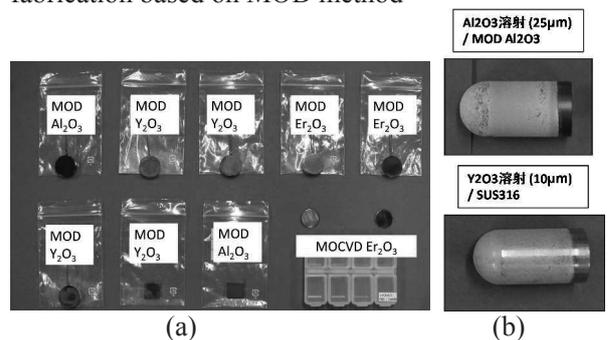
Fig. 3 (a) Specimens coated by MOD method, (b) Specimens have duplex coating by MOD method and APS
