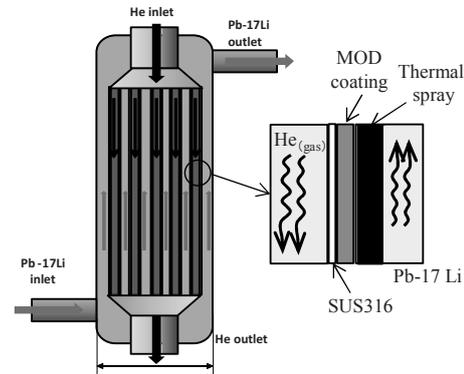
Fig. 1 Application of ceramic coating on heat transfer tube in heat exchanger
