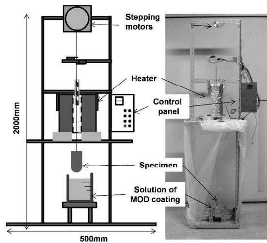
Fig. 2 Experimental apparatus for ceramic coating fabrication based on MOD method
