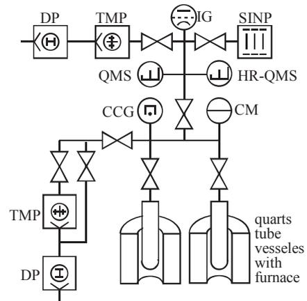
Fig.1 Tritium release apparatus for TDS and baking experiment. It consists of two turbo molecular pump (TMP), two dry pump (DP), a quadrupole mass spectrometer (QMS) and a high-resolution QMS(HR-QMS), a sputter ion noble pump (SINP), a capacitance manometer (CM), a cold cathode gauge (CCG), an ion gauge (IG) and two quartz tube vessels with furnaces.
