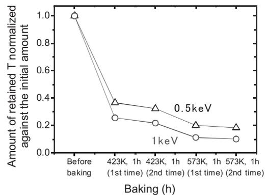
Fig.2 Tritium decontamination by thermal baking at under vacuum condition.
