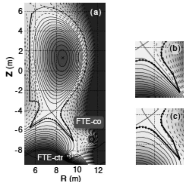
Fig. 1. Example of the FTE divertor for a DEMO reactor with  $I_p = 15 \text{ MA}$ . FTE currents are  $I_c = +4 \text{ MA}$  and  $-4 \text{ MA}$ . Rate of the FTE,  $G_{\text{FTE}} = 2.7$ , is evaluated by comparing (b)  $I_c = 0 \text{ MA}$  and (c)  $I_c = 4 \text{ MA}$ .
