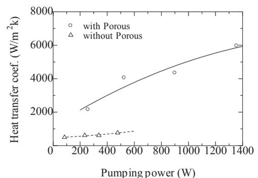
Fig. 2 Heat transfer performance for pumping power
