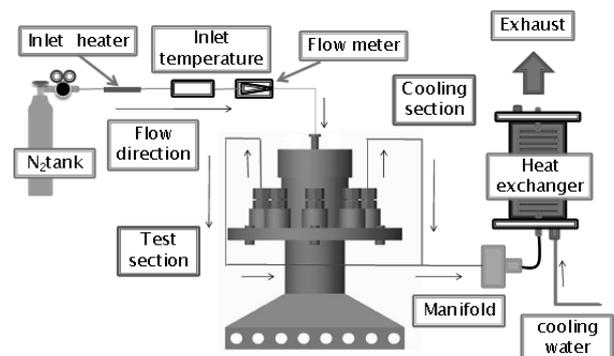
Fig.1 Experimental set up of gas cooling
