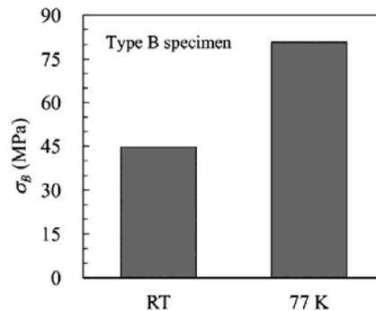
Fig. 4. Through-thickness tensile strength.
