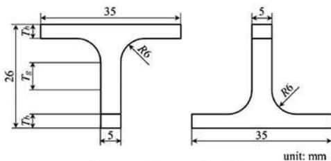
Fig. 1. Specimen configuration.
