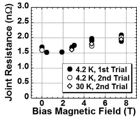
Fig. 1. Joint resistance as a function of bias magnetic field for the 100-kA-class HTS conductor.
