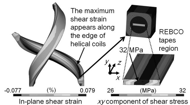
Fig. 2. Distribution of in-plane shear strain in helical coils (left figure) and distribution of  $xy$  component of shear strain in the REBCO tape region (right figure).
