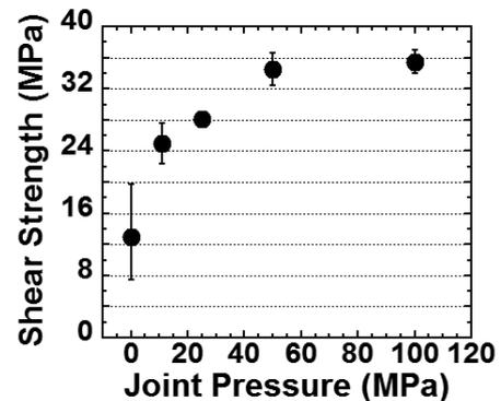
Fig. 3. Shear strength of joint as a function of joint pressure obtained in tensile shear test of a mechanical lap joint of GdBCO tapes.
